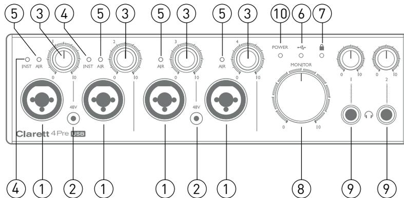
The front panel includes input gain and monitoring controls as well as four of the input connectors for Mic, Line and Instrument signals.
