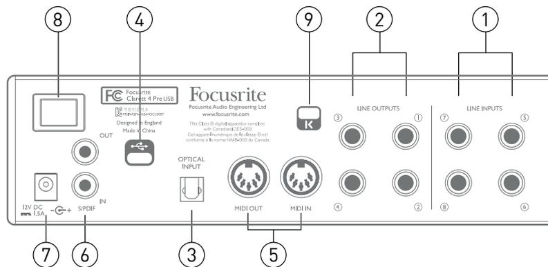
1. **LINE INPUTS 5 to 8** – four balanced analogue line inputs for Channels 5 to 8, on ¼” TRS jack sockets. Connect further line level signals here using ¼” TRS (balanced) or TS (unbalanced) jack plugs.
