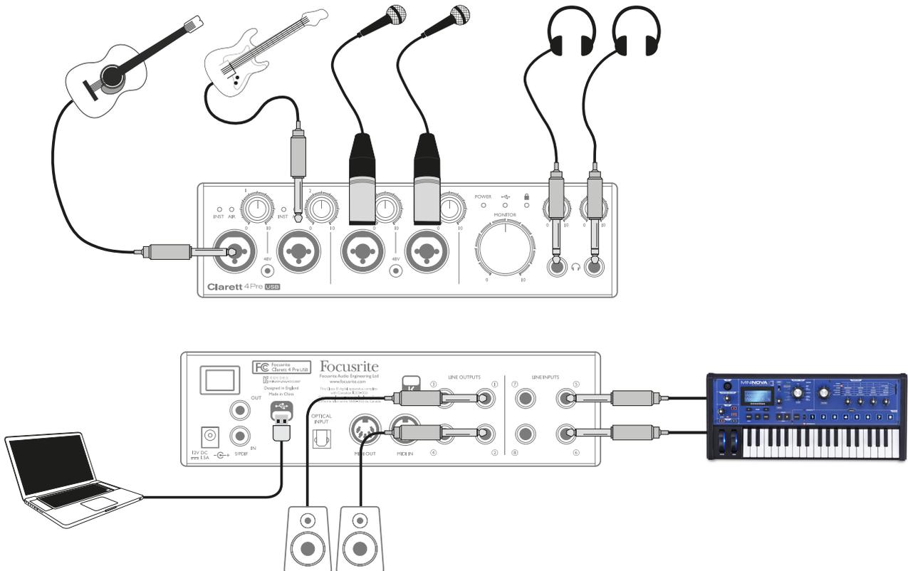
This setup illustrates a typical configuration for multitrack recording with DAW software on your computer.
