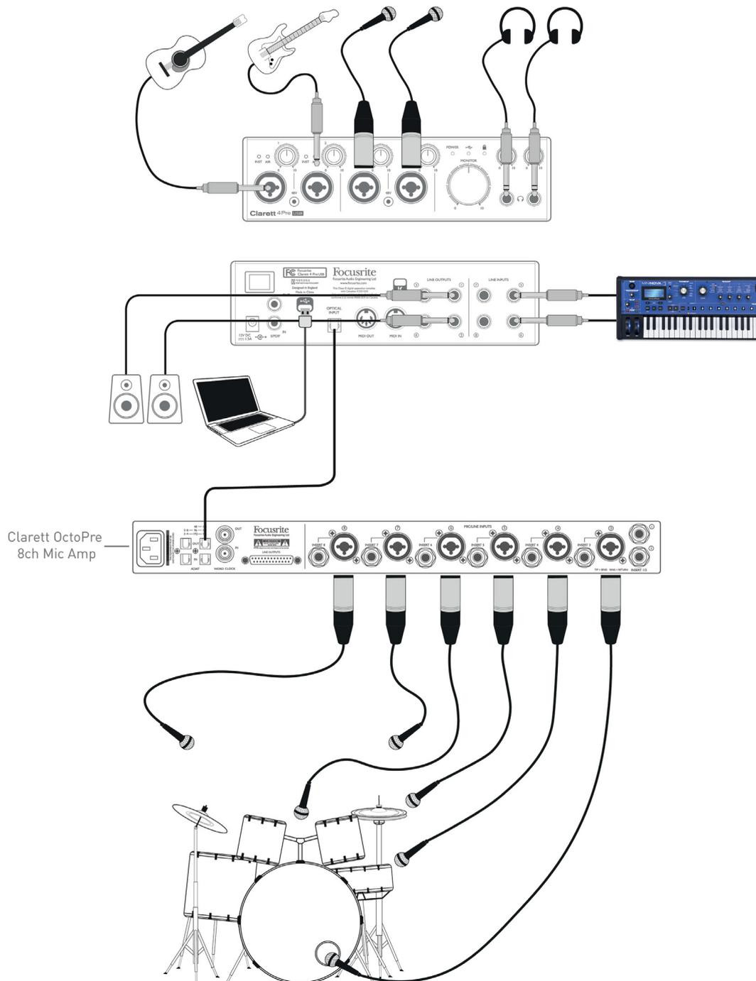
The Clarett OctoPre's **OPTICAL OUT** port is connected to the Clarett 4Pre USB's **OPTICAL IN** port with a single TOSLINK optical cable. The two devices must be synchronised to ensure audio passes cleanly, without clicks and pops. This can be achieved by selecting ADAT as the clock source on the
